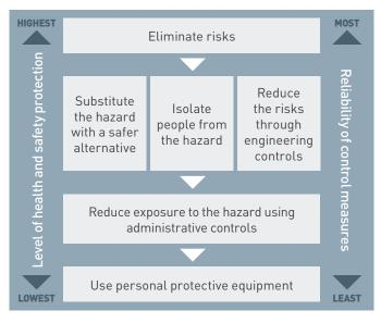
Figure 3: The Hierarchy of Control.<sup>18</sup>
