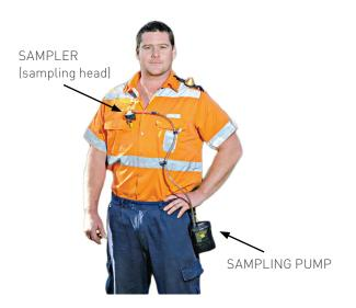
Figure 4: Personal dust sampler
